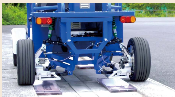
Third-generation in-wheel motor with dynamic wireless charging
